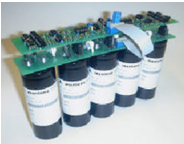
Fig. 15. Supercapacitors assembled in series [1].
