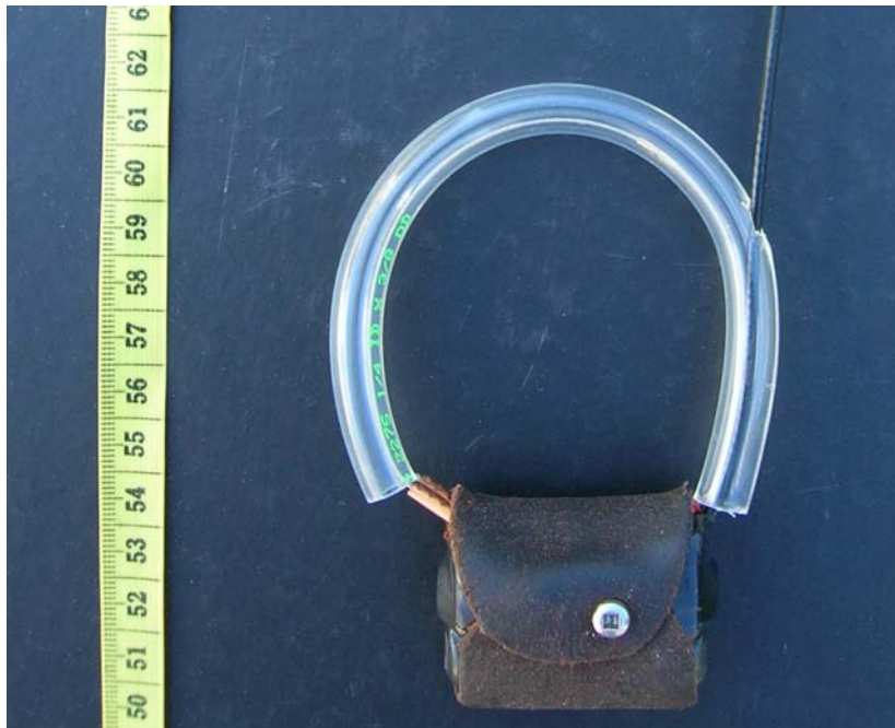
Figure 2.2 : Tygon tubing system used to attach radio transmitter to North American porcupines in Parc National du Bic, Québec, May 2000-May 2005. Note that the metallic part (cramp) used to close the collar is visible on the picture but was inserted into the Tygon after the collar was adjusted around the porcupine's neck. Photo by S. Descamps.
